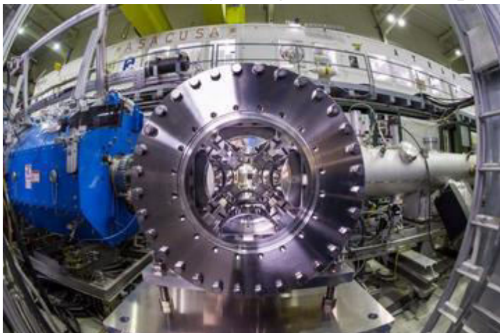
Photograph of the quadrupole triplet lens used to focus the antiproton beam into a helium target. Credit: CERN
