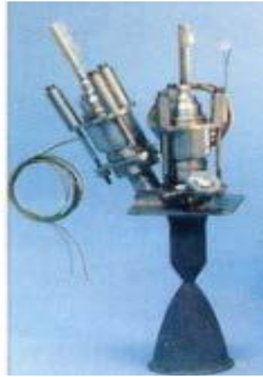
8 nos. of 22 N AOCS (Attitude & Orbit Control System) Thrusters
