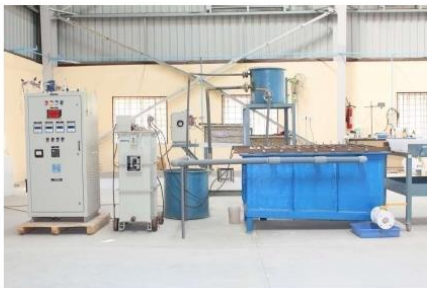
Copper Electrowinning system
