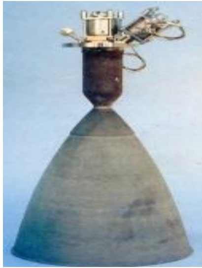
440 N LAM (Liquid Apogee Motor) as the main engine
