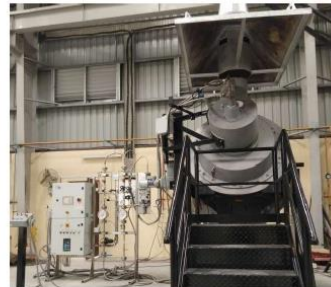
TBRF erected with fume hood
